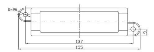
Insulating Body : Nylon With Glass Fiber / PC Applicable : For ANL 25A~200A
