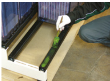
Fig. 5-13: Greased support profiles
