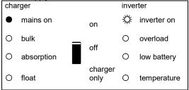
The AC voltage on AC-in-1 or AC-in-2 is switched through, but the load demands more current than the mains can supply. The inverter is now switched on to supply additional current.
